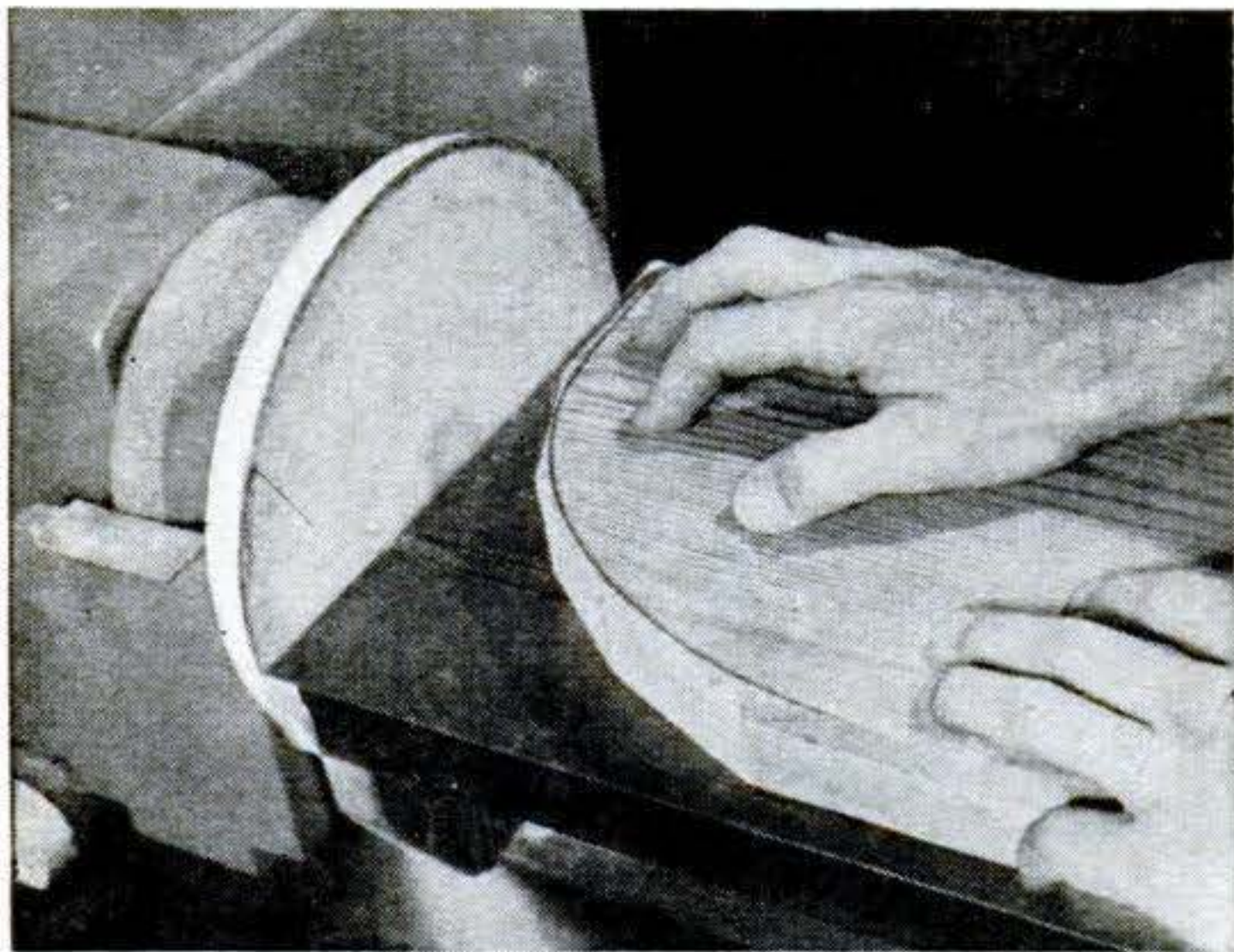
DISK SANDER speeds work. Corner was rough-sawed to shape, then rounded on sander.
